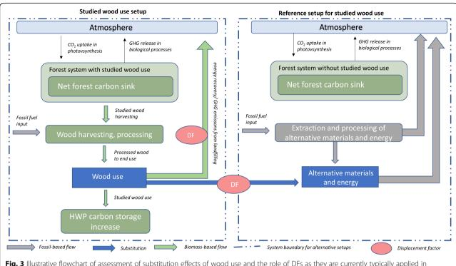
Fig. 3 Illustrative flowchart of assessment of substitution effects of wood use and the role of DFs as they are currently typically applied in scientific literature
