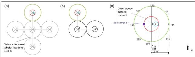
Fig. 4 Plot and subplot configurations (a) Sal, Hill, Village and Coastal zones, (b) Sundarban zone and (c) subplots. The number of subplot locations in the Sundarban zone was limited to three to ensure plot measurements to be completed within one day
